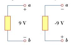
(a) point a is at a potential of  $v_{ab}$  volts higher than point b, or
